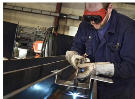
Torch cutting a steel plate; Fixing an engine part on board a fishing vessel (opposite, left); Partial view of new workshop hall under construction, May 2018 (opposite, right).
